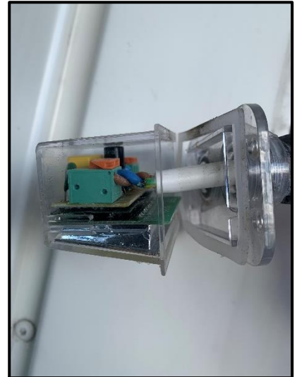
3. Slide the plastic lid back up the cable careful of rubber seal
