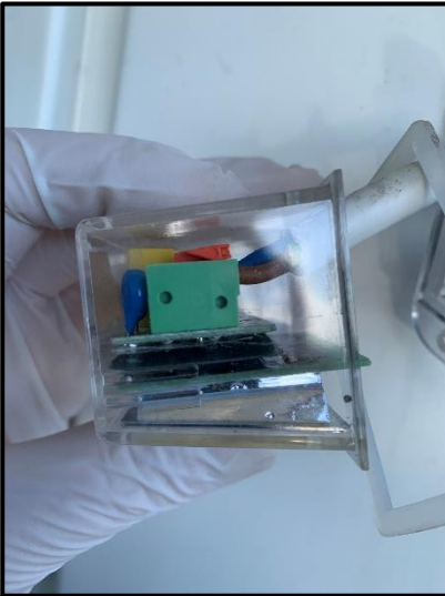
10. Slide bulb back into case. Fitting circuit board into slots
