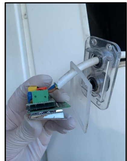
9. Slide over the rubber seal then fit reflector and hold in place
