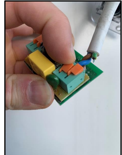
6. Slide clips backwards to release wires (Can be quite stiff)
