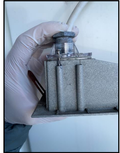
12. Fit bulb case back into light surround and refit screws
