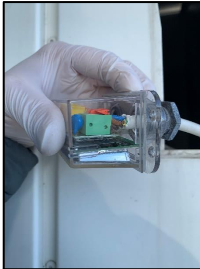
Refit plastic lid making sure to seat the rubber seal correctly
