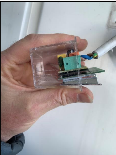
Slide lightbulb out of case being careful not to drop reflector
